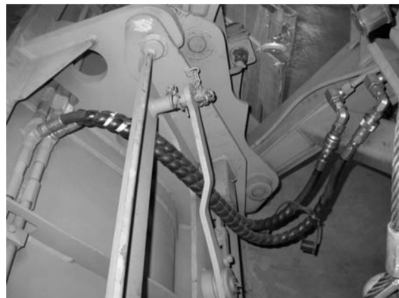
ROUTE HOSES THROUGH QUICK-HITCH FRAME AS SHOWN
